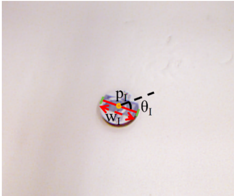
Figure 1. Schematic diagram of the grasping configuration of the parallel gripper
