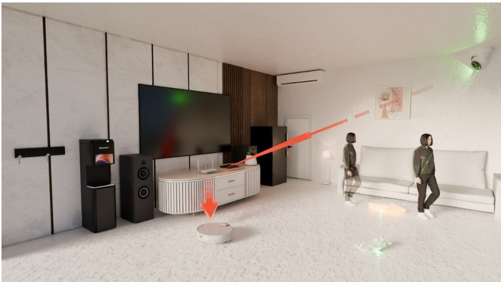
Figure 1: Web camera detecting dirt/trash and human movement communicates with vacuum robot
