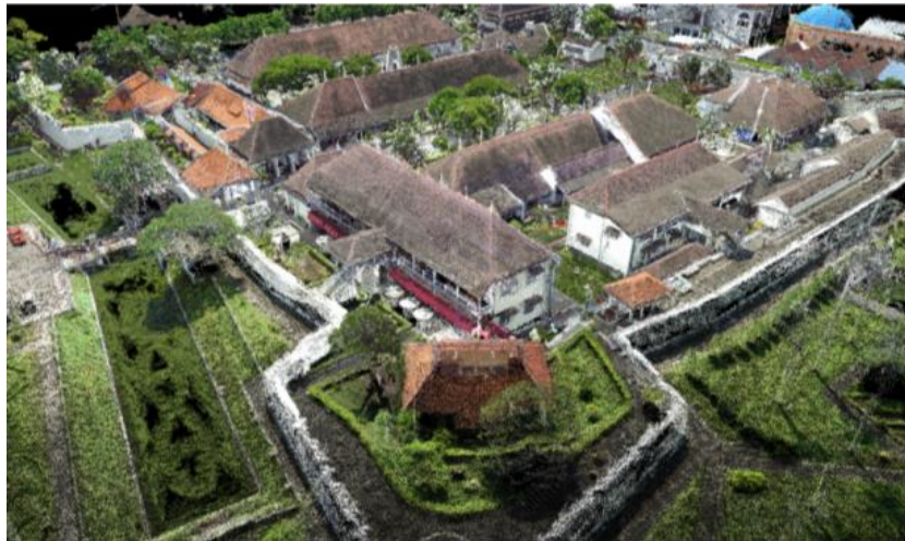
Figure 1. Integration of TLS and UAV pointclouds data by using Iterative Closest Point (ICP) algorithms
