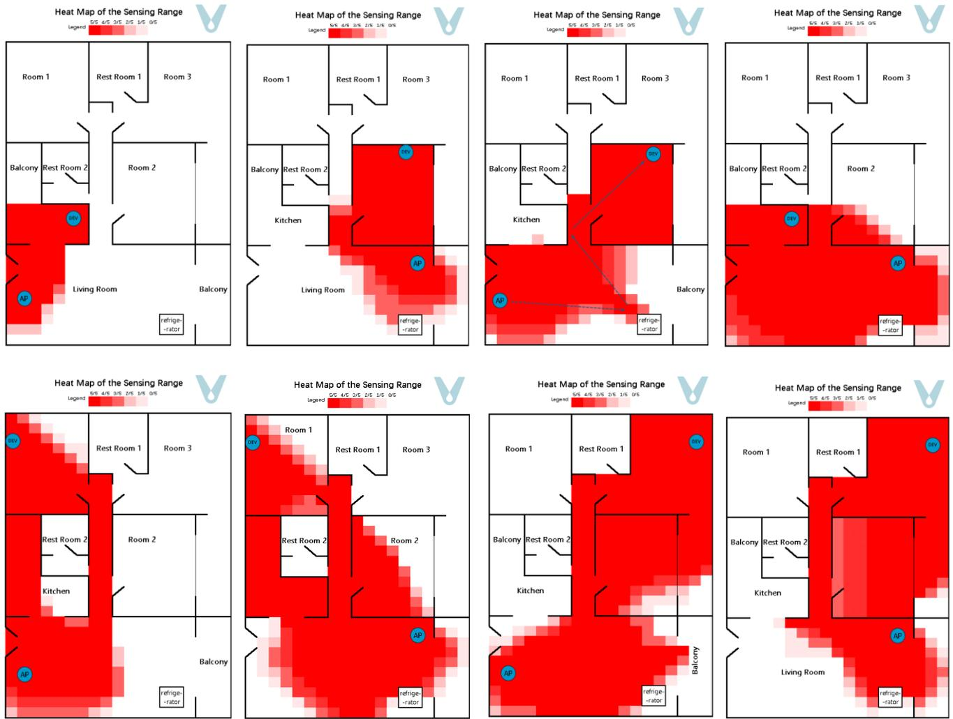
**Figure 11.** Sensing heat map of the multipath fading scenario (single terminal)
