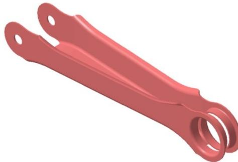
**Figure 9.** Schematic diagram of the control arm with an upward-opening structure
