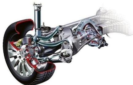
**Figure 1.** Schematic diagram of the five-link rear suspension
