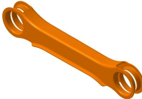
**Figure 8.** Schematic diagram of the control arm with bushings press-fitted on both sides
