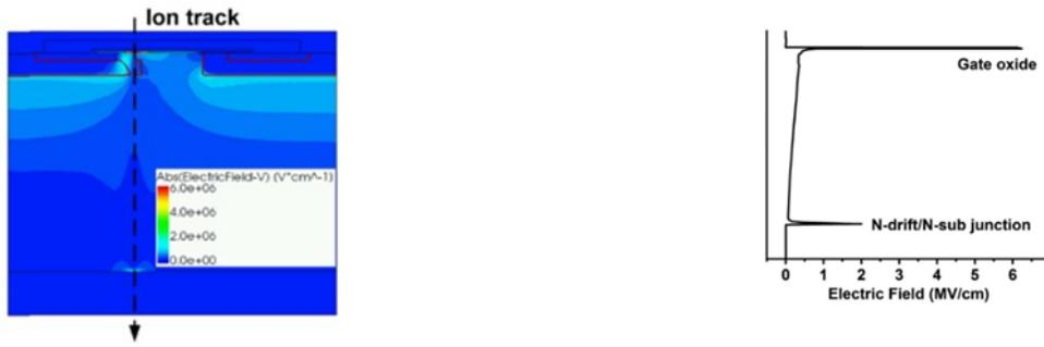
(a) Ions attack the gate oxide position
